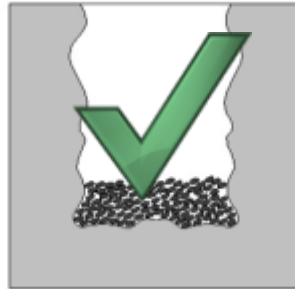
with drainage bed (e.g. loose subsurface)
