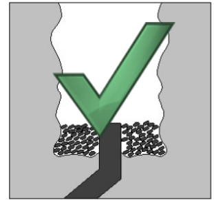
with drain pipe (e.g. solid subsurface)
